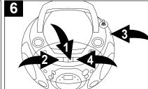
If you wish to listen to your recording immediately, press the cassette REWIND (▶▶) button ① until the tape rewinds to the beginning, then press the STOP/EJECT (■▲) button ②. Slide the FUNCTION switch ③ to the TAPE position and press the PLAY (◄) button ④ to begin playback.
