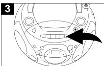
Open the Cassette Door and insert a good quality blank cassette tape into the slots on the door, with the open end facing up and the full reel on the right-hand side. Close the Cassette Door.
