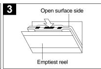
Insert a pre-recorded cassette into the slots in the Cassette Door with the open end facing up and the full reel on the right side. Close the cassette door.
