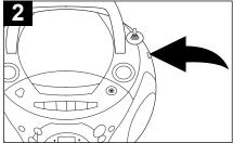
Slide the FUNCTION switch to the CD position; the POWER ON indicator will light.
