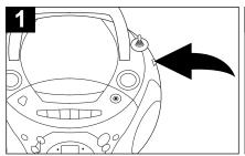
Slide the FUNCTION switch to the CD position; the POWER ON indicator will light. Insert a CD as described in the TO INSERT A CD section on page 6.
