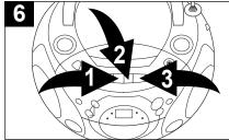
To advance or rewind the tape rapidly, press either the F.FWD (◀◀) ① or REWIND (▶▶) ② button. When you reach the desired point, press the PLAY (◄) button ③ to resume normal playback.
