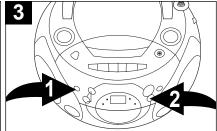
Press the REPEAT button ① once, the REPEAT indicator will blink and the unit will play the selected track over and over until the STOP (■) button ② is pressed.
