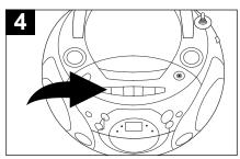
To avoid recording unwanted material, such as radio commercials, use the PAUSE (II) button to stop the recording temporarily. Release the PAUSE (III) button to begin recording again.
