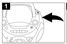
Slide the FUNCTION switch to the TAPE position.
