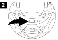
Press the STOP/EJECT (■▲) button to open the Cassette Door.
