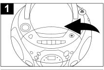
Press the CD Door OPEN/CLOSE area to open the CD compartment door. Place a CD on the center spindle, with the printed label side facing up. Close the CD compartment door.
