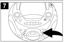
When the disc is through playing, it will stop rotating. Press the STOP (**■**) button to stop the disc before it is finished.
